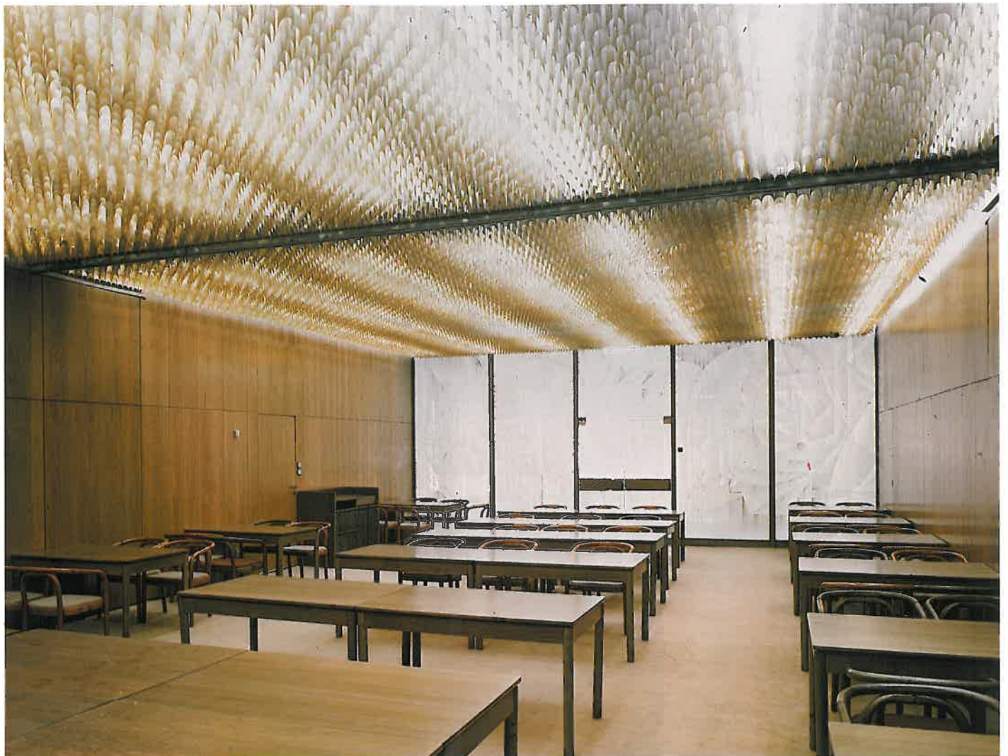
Two committee rooms. A virtue has been made of the uneven flashing of the leaf-lite ceiling, due to limited head-room, as it relieves the monotony of the ceiling. In the room shown below a Programme 2 ceiling has been installed.
